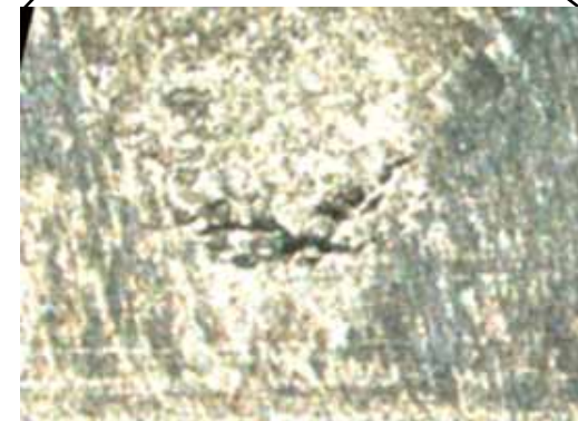
75-mil Crack Cluster (Maximum Crack Length 50 mils)
