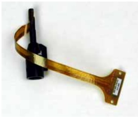
Mandrel Assembly with interchangeable MWM-Arrays
